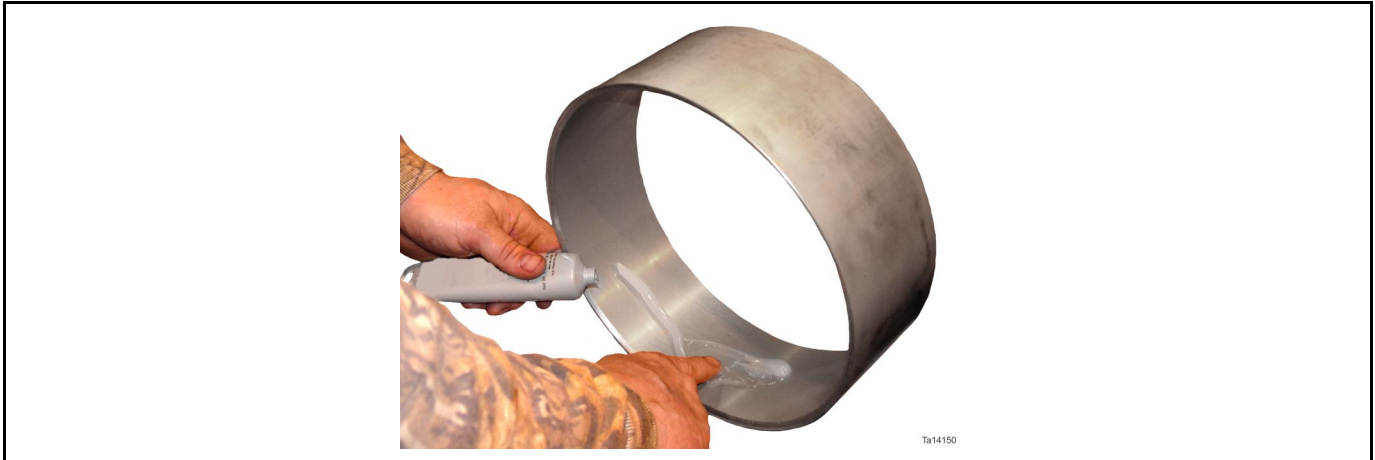
Figure 76: Lubrication of inner housing
