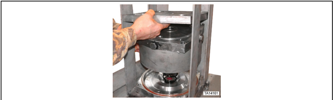
Figure 84: Placement of press plate into press for final assembly of inner actuator
