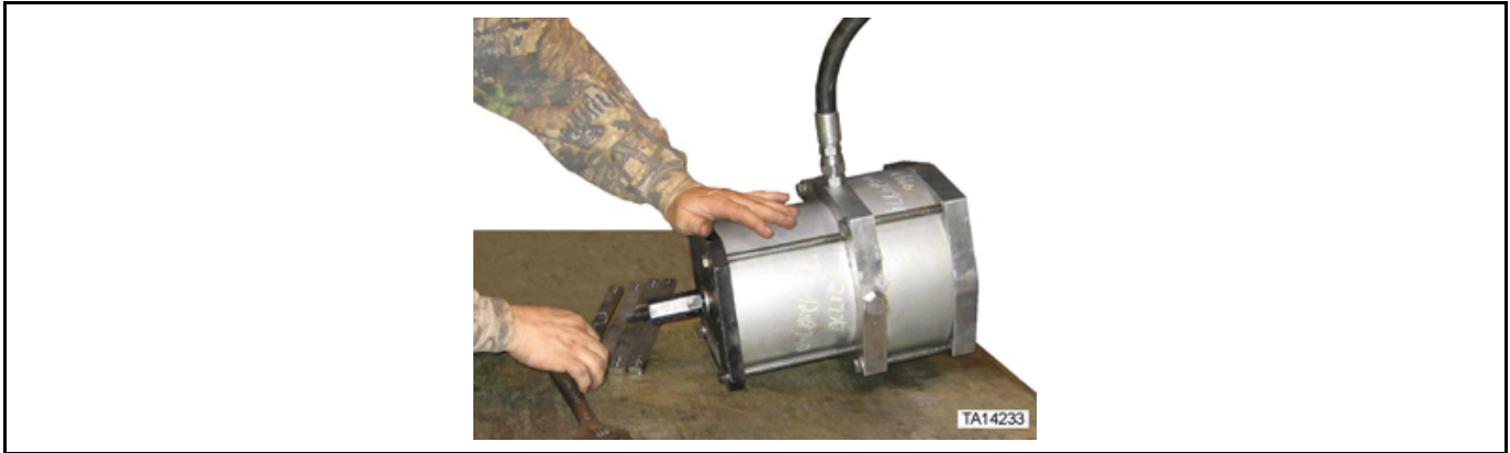
Figure 99: Use of jack bolt to release park brake to test actuator operation
