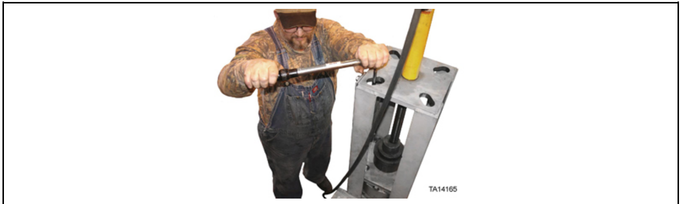
Figure 88: Installation of bolts securing inner canister components
