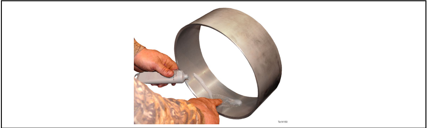
Figure 90: Lubrication of inner housing
