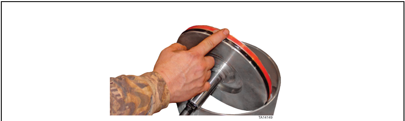
Figure 75: Lubrication of seal and wear ring
