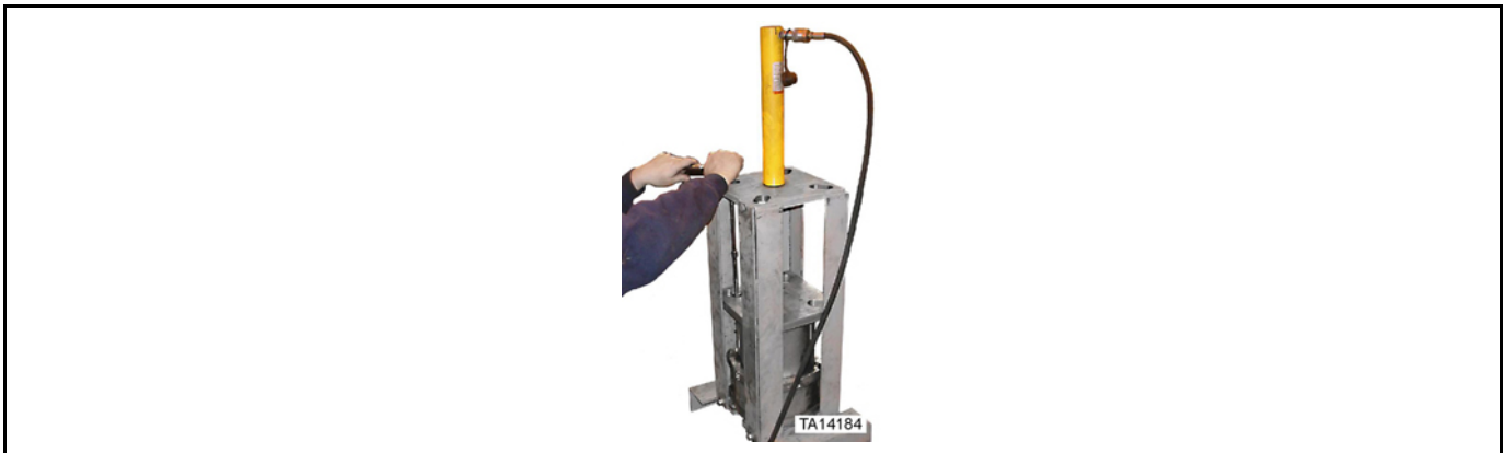
Figure 64: Removal of bolts securing end cap (1 of 2)
