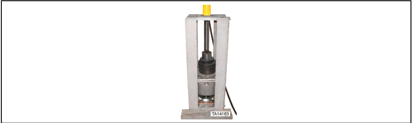
Figure 86: Pressing inner canister for final assembly (1 of 2)
