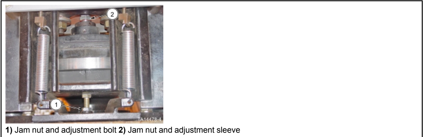
Figure 45: Brake pad adjustment points top side view
