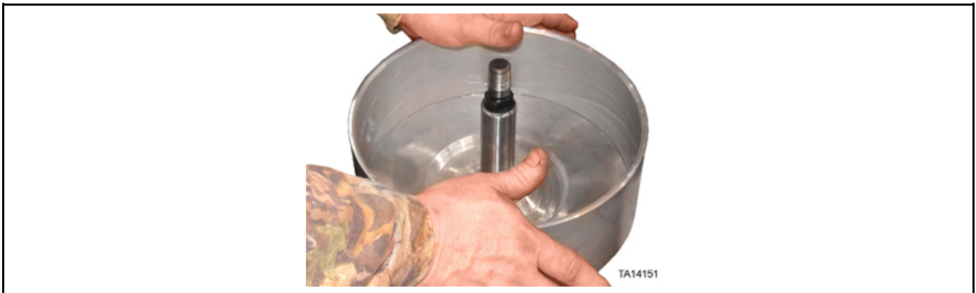
Figure 77: Installation of piston into inner housing
