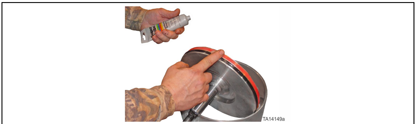
Figure 89: Lubrication of seal and wear ring
