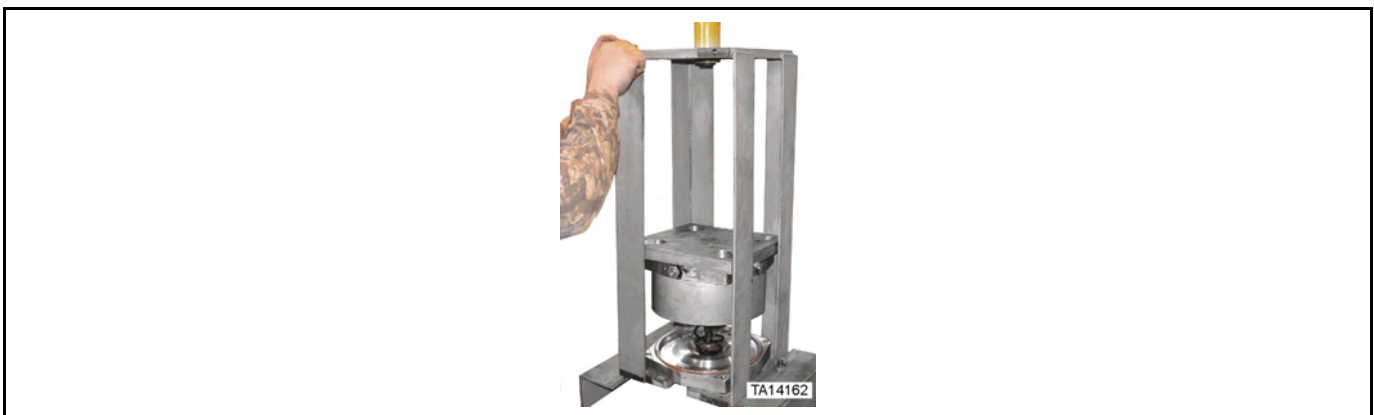
Figure 85: Installation of safety plates prior to final assembly of inner canister
