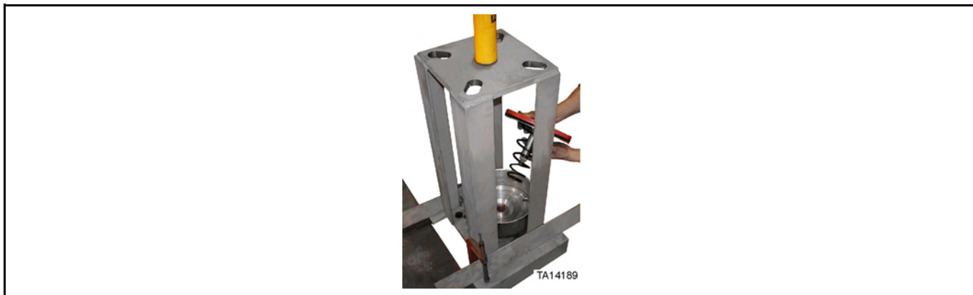
Figure 68: Removal of inner spring and piston
