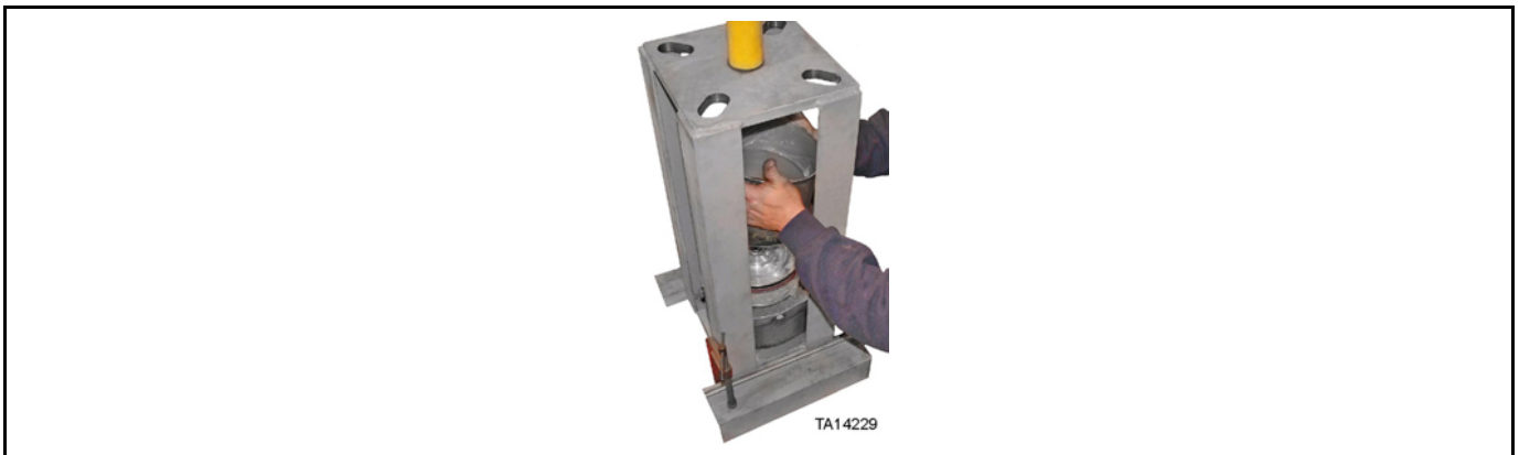
Figure 93: Installation of outer housing
