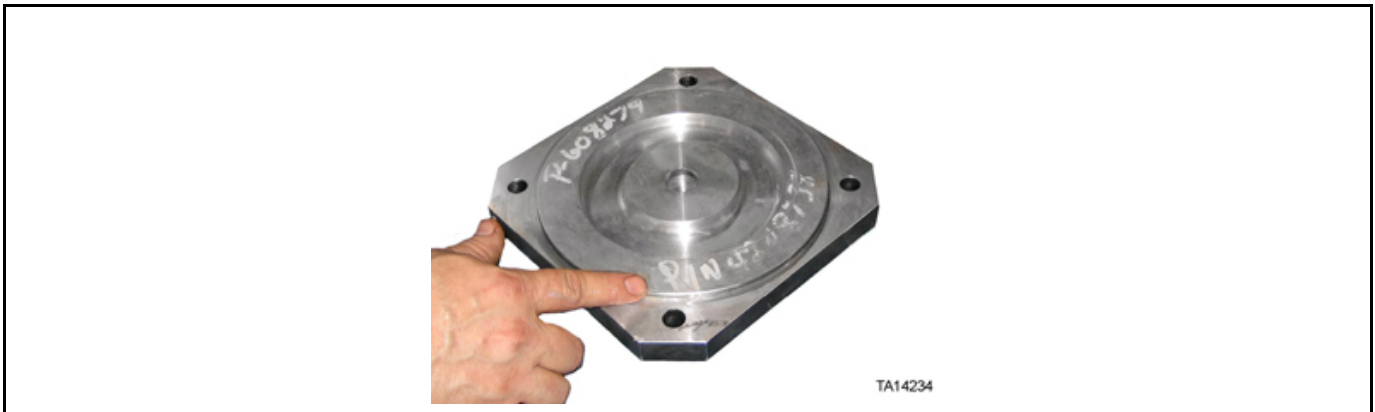
Figure 91: Lubrication of end cap installation of O-ring
