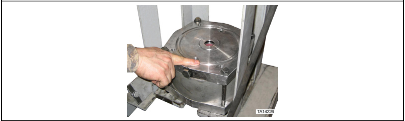
Figure 92: Lubrication of inner end cap for installation of O-ring
