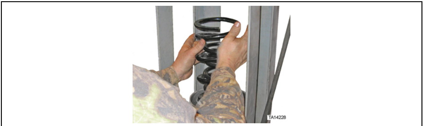
Figure 95: Installation of spring assembly into housing
