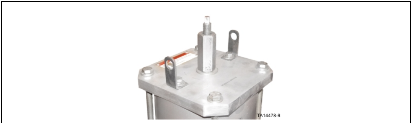
Figure 40: View of jack rod installed in brake cylinder
