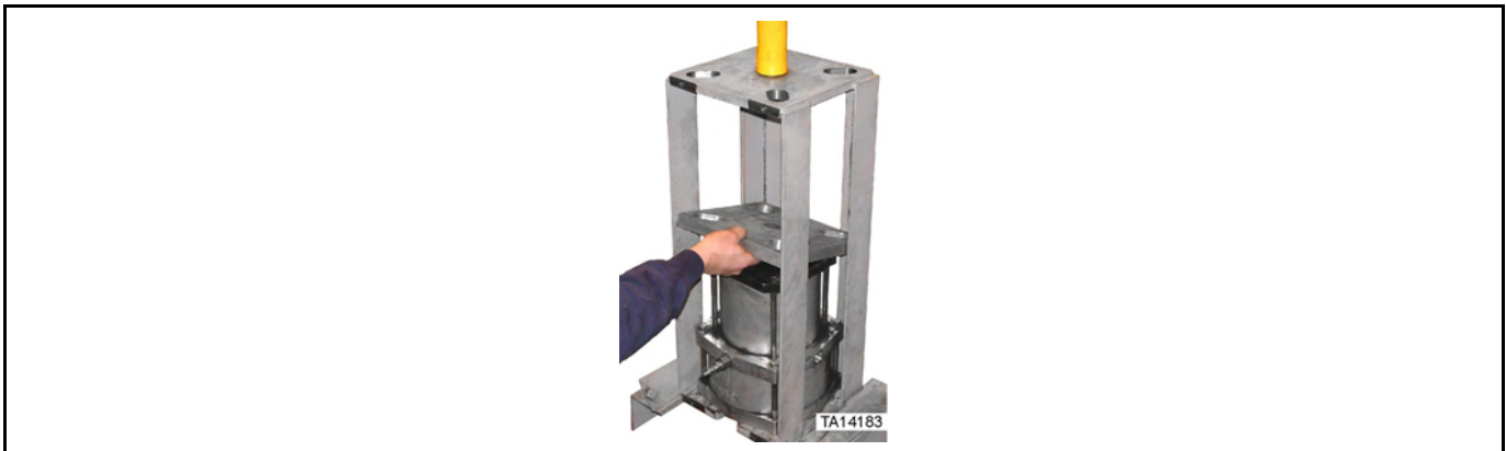
Figure 62: Placing press plate into press
