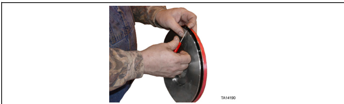
Figure 69: Removal of seals and wear rings (1 of 2)
