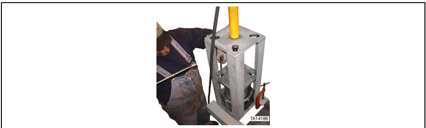
Figure 65: Removal of bolts securing end cap (2 of 2)
