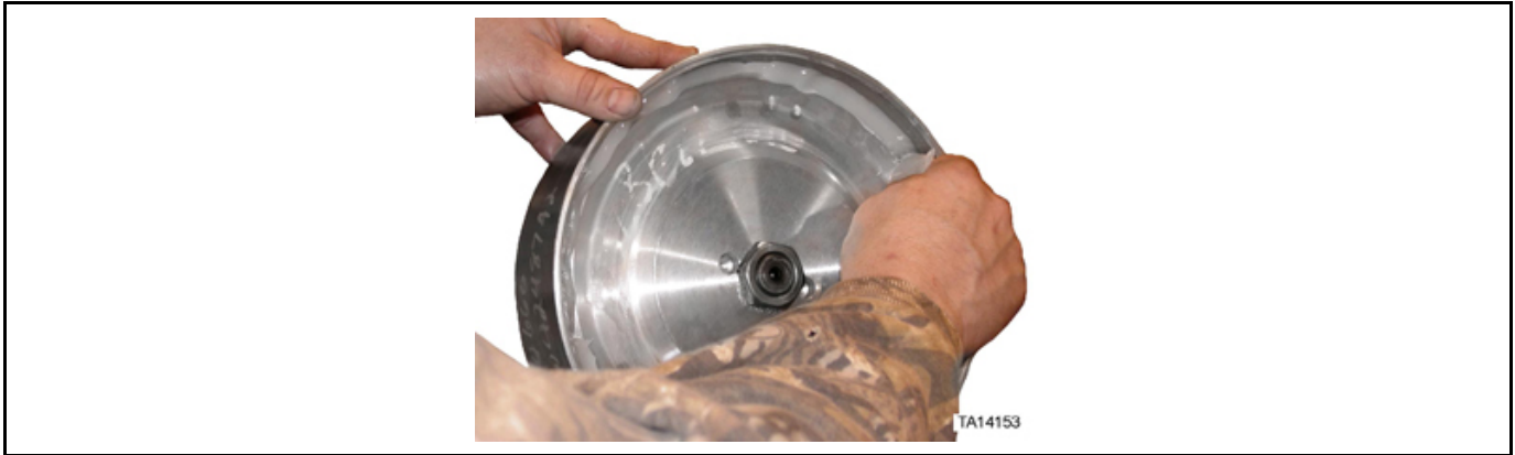
Figure 78: Lubrication of piston in inner housing
