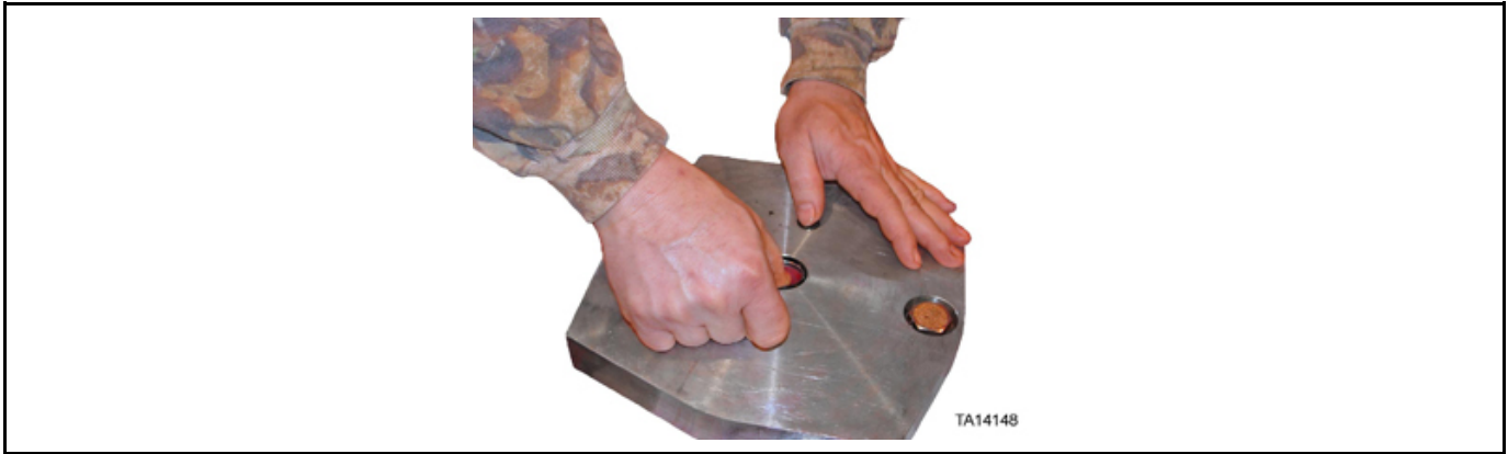
Figure 72: Installation of O-ring to end cap
